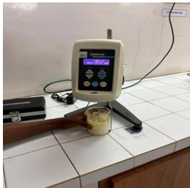
Figure 16. Viscosity determination using a Brookfield viscometer.
