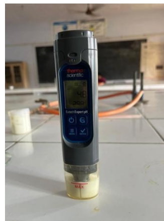
Figure 15. pH determination of the formulated nanoemulgel using a calibrated digital pH meter.
