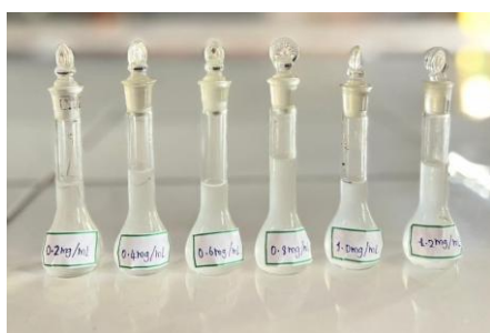
Figure 18. Dilution of the nanoemulgel sample prior to spectrophotometric measurement for SPF determination.
