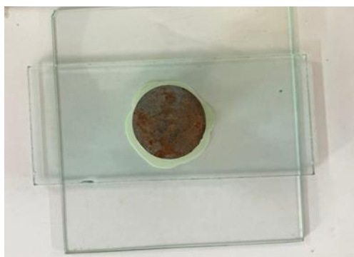
Figure 17. Spreadability test setup using the parallel-plate (slip-and-drag) method.
