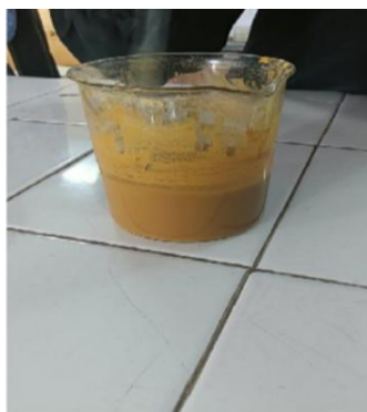
Figure 7. Zinc(II) mixed-ligand complex of 5-nitro-8-hydroxyquinoline and L-threonine (final product).
