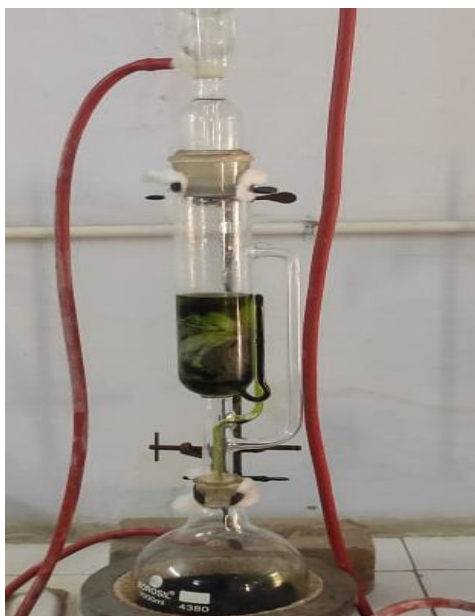
Figure 1. Extraction of Carica papaya Leaves Soxhlet Apparatus
